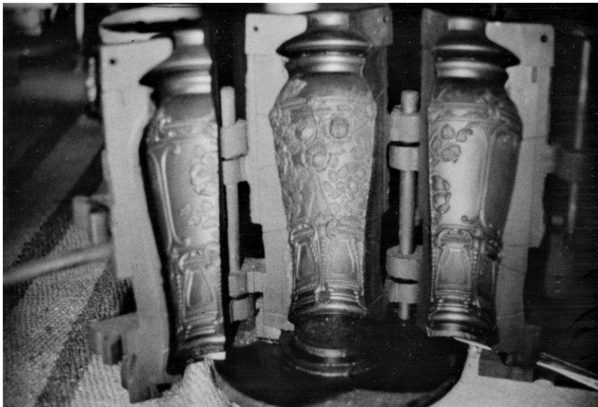
Figure 4: Photo of Goofus Jar Mould. J. Edward Pfeiffer Manuscript Collection, Batsto State Park, NJ. Collection now resides in the New Jersey State Archives, Trenton, NJ.
